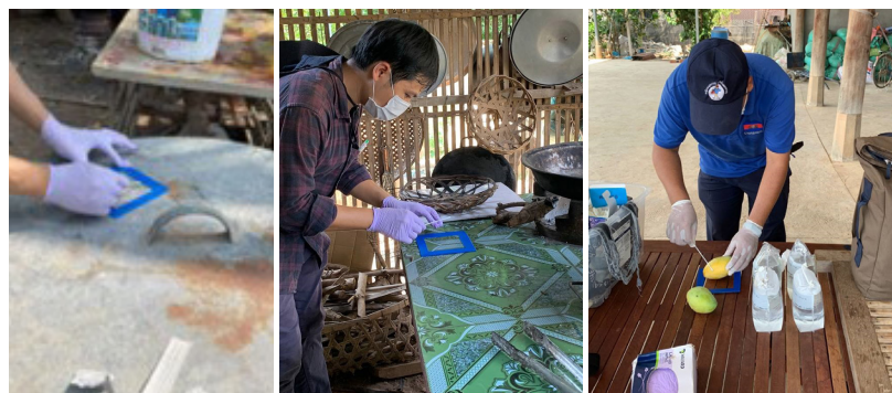
Sampling (left to right) a water container, a kitchen table, and a mango. Photo credit: Tetra Tech
