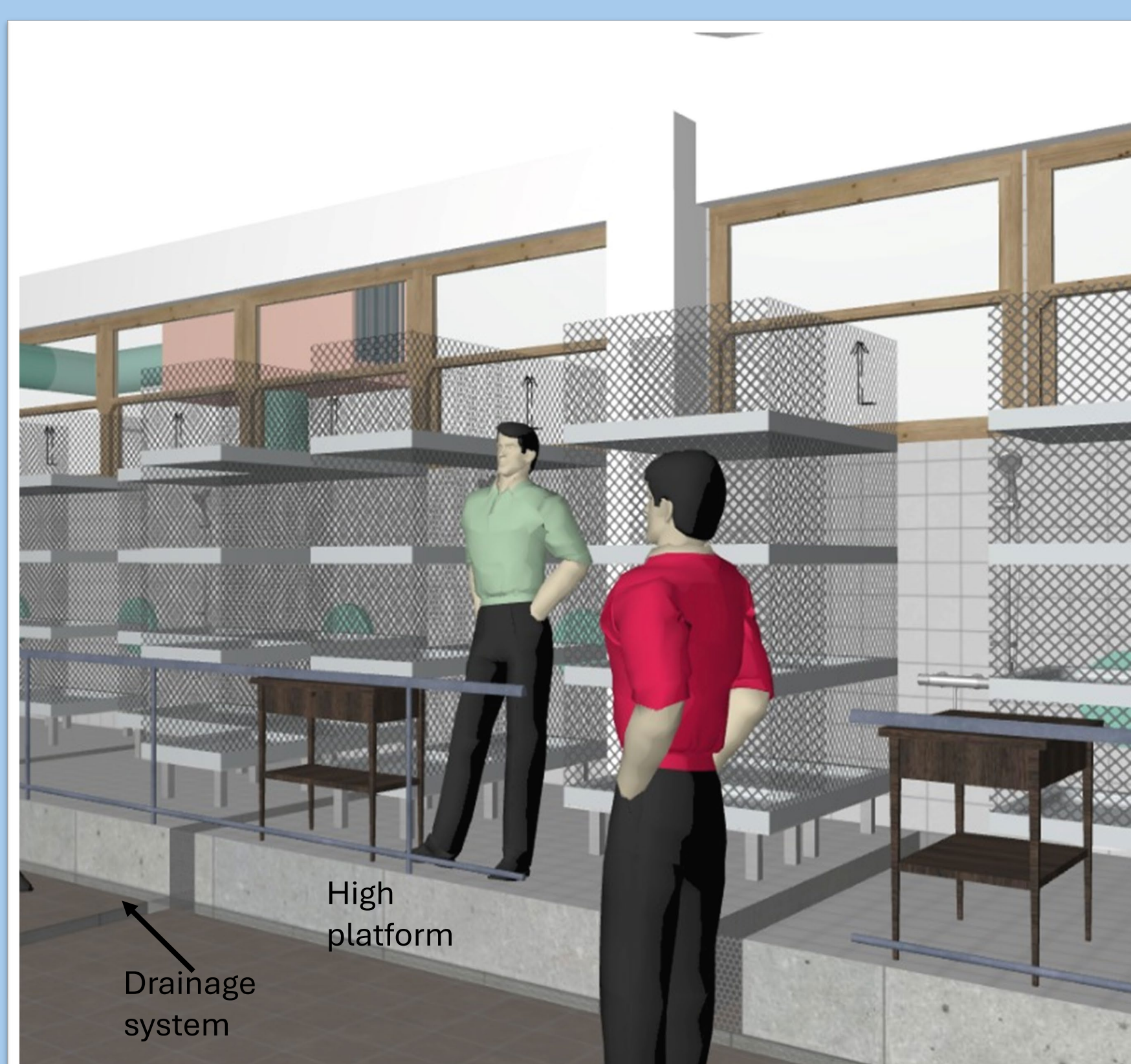
Figure 5: High platform and drainage system
