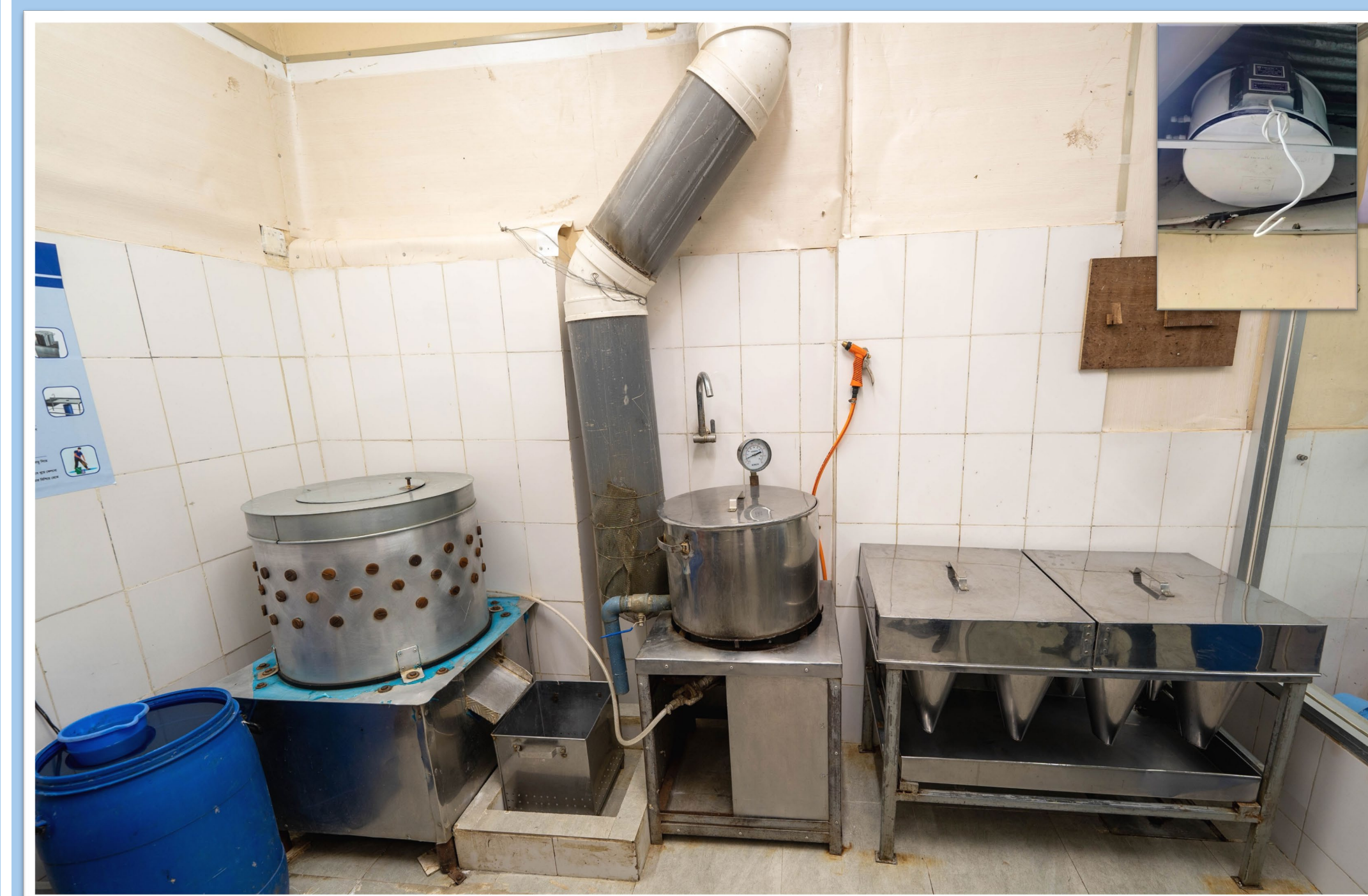
Figure 8: Slaughtering cone, scalding arrangement, and defeathering machine with the lid
